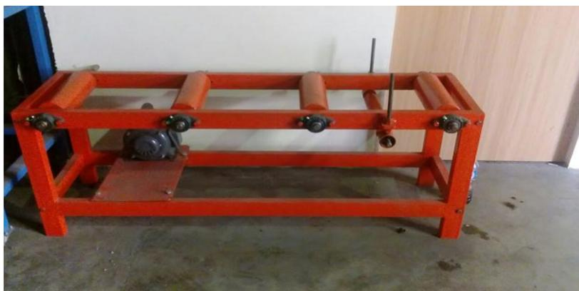
Gambar 3.8. *Roller belt conveyor*
