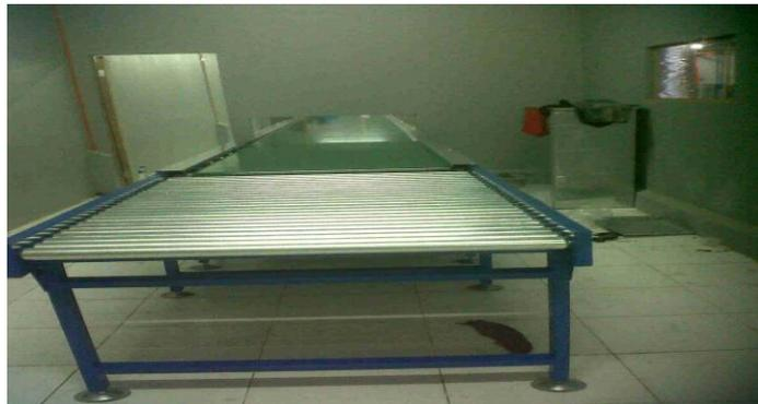
Gambar 2.5. *Conveyor roller*
