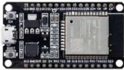
Gambar 2. 3 Node MCU ESP32 Sumber : Arrahma & Mukhaiyar., (2023)
