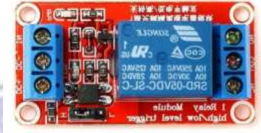
Gambar 2. 10 Relay 1ch 5V opto
