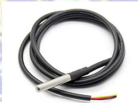
Gambar 2. 9 Sensor Suhu Ds18b20
