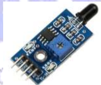
Gambar 2. 8 Sensor api (Flame)
