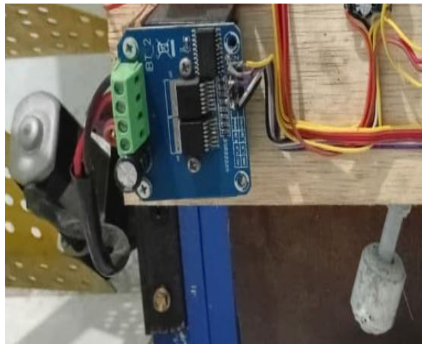
Gambar 4.12 Power window bergerak sesuai kendali motor bts7960
