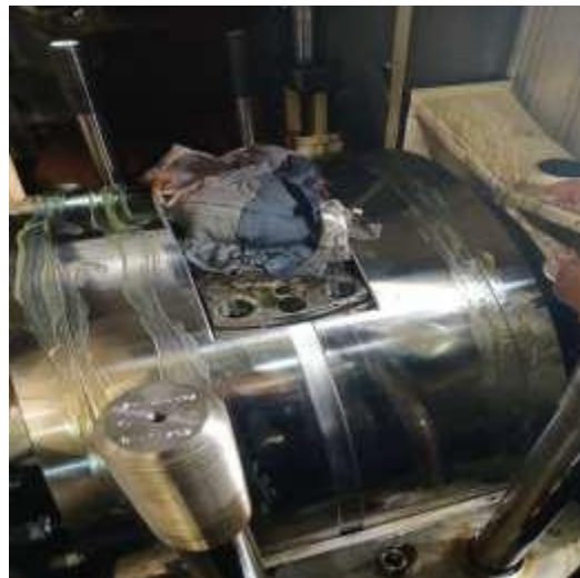
Gambar 4.1 Pengukuran Clearance Bearing Crosshead (PT. WSI)
