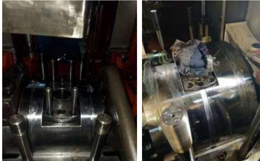
Gambar 4.7 Pengukuran Clearance Bearing Crosshead (PT.WSI)
