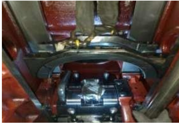
Gambar 2.8 Sistem Crosshead (P.T Waruna Shipyard Indonesia)
