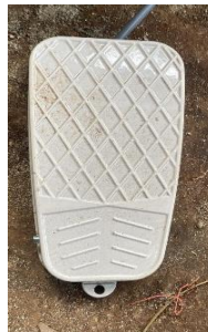
Gambar 3.11 Foot Switch 10A 250 VAC
