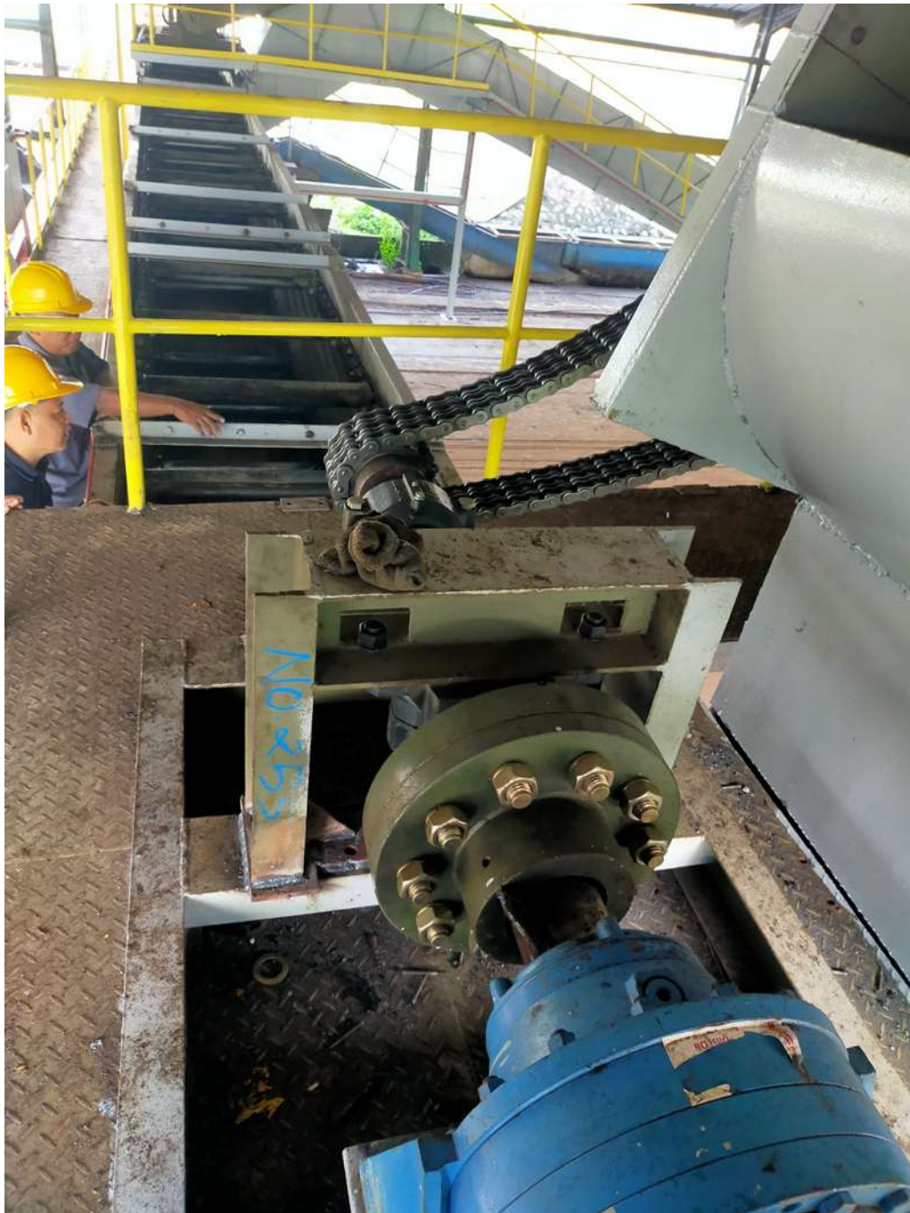
Lampiran 3. Motor dan Couplean ke chain conveyer FFB
