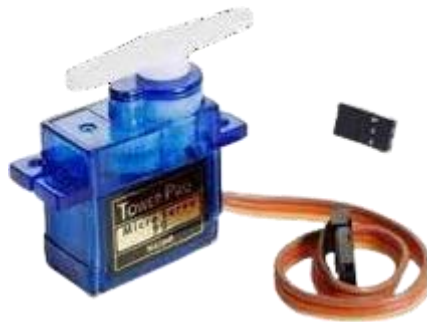
Gambar 2.6 Motor Servo SG90
