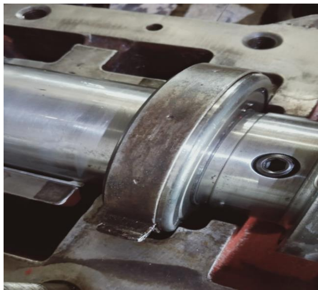
Gambar 2.9 Thrust Bearing (PT.Sodetan Pom,2024)
