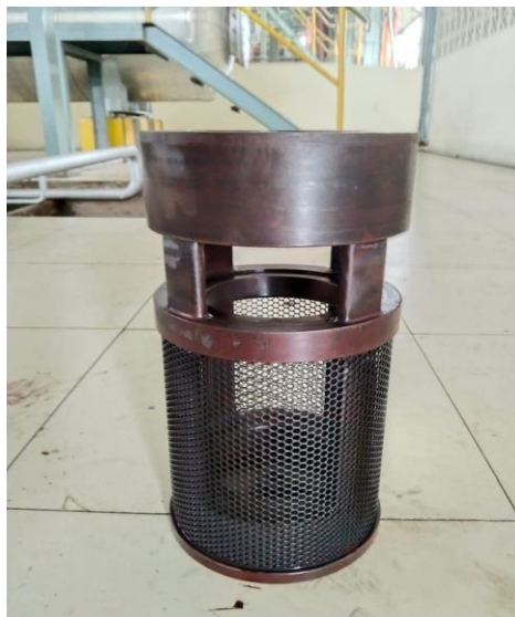
Gambar 2.20 Steam Strainer (PT.Sawita Estate,2024)
