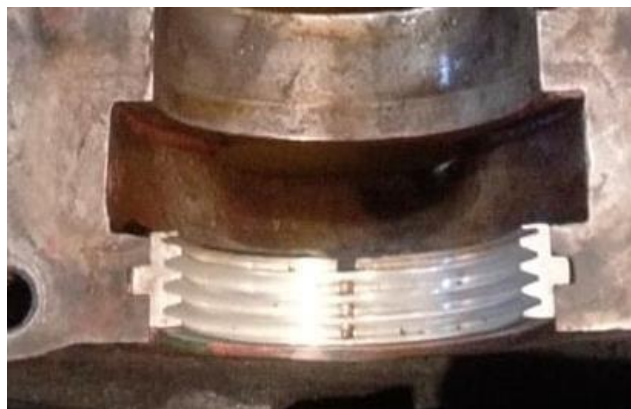
Gambar 2.14. buffle Oil (PT.Sodetan Pom,2024)
