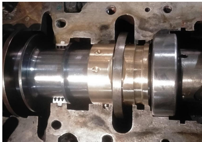
Gambar 2.8 Journal Bearing (PT.Sawita Estate,2024)
