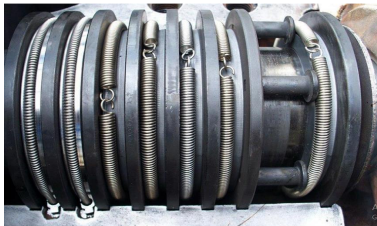
Gambar 2.4 carbon ring (PTPN III Aek Raso,2024)
