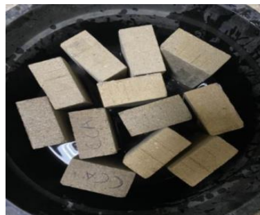
Gambar 4.10: Proses perendaman batu bata
