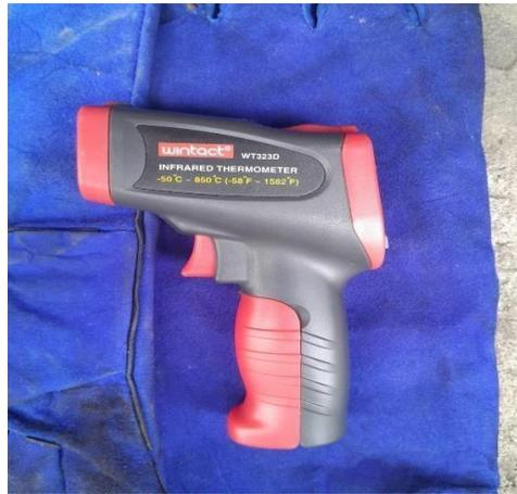
Gambar 2. 14 *Thermometer infrared*
