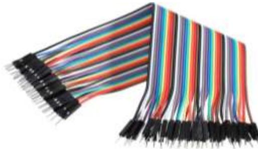
Gambar 2.11 Kabel Jumper
