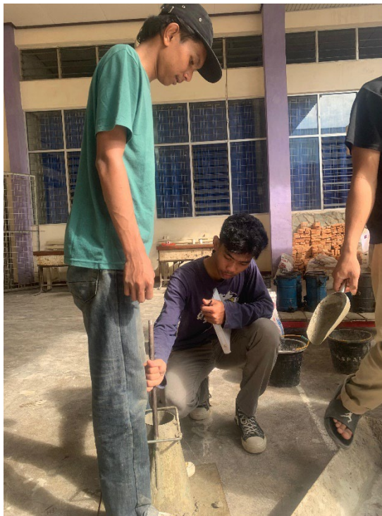
Gambar L. 6: Pengujian Slump Test
