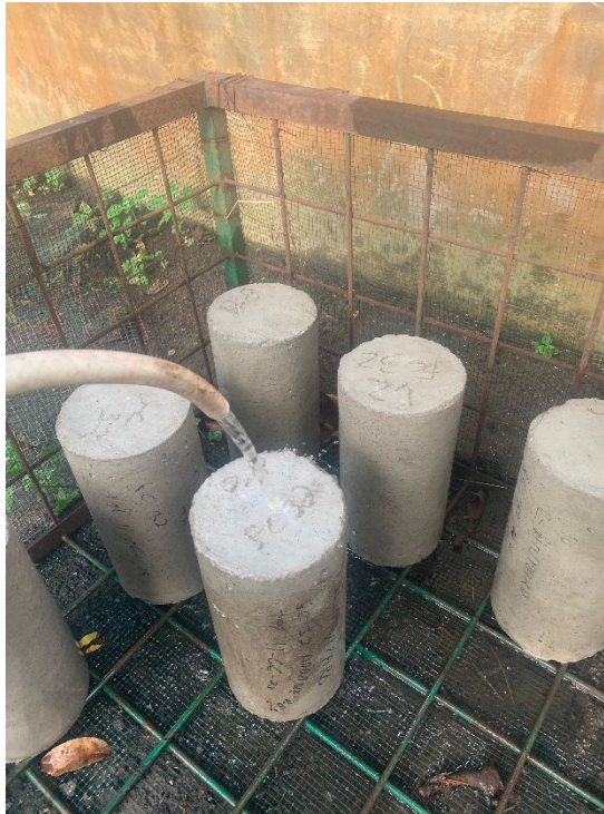
Gambar L. 11: Curing Siram Beton Segar
