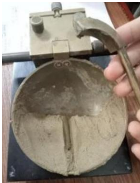
Gambar 4.3: Uji Plastisitas Tanah Galong.
