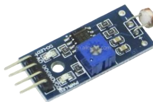
Gambar 2.5 LDR sensor (Sumber https://38-3d.co.uk )
