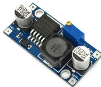
Gambar 2.6 Modul LM2596 DC-DC Step Down (Sumber https://digiwarestore.com )
