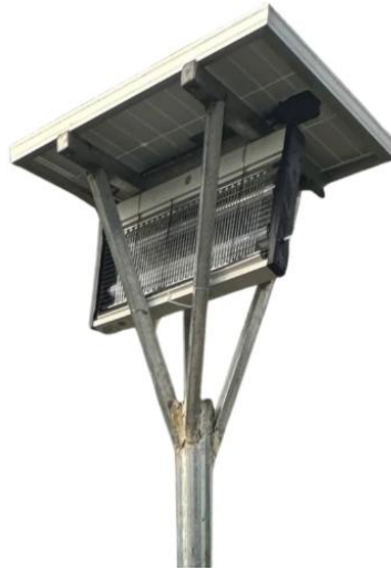
Gambar 4.1 Smart Anopheles Trap Lamp
