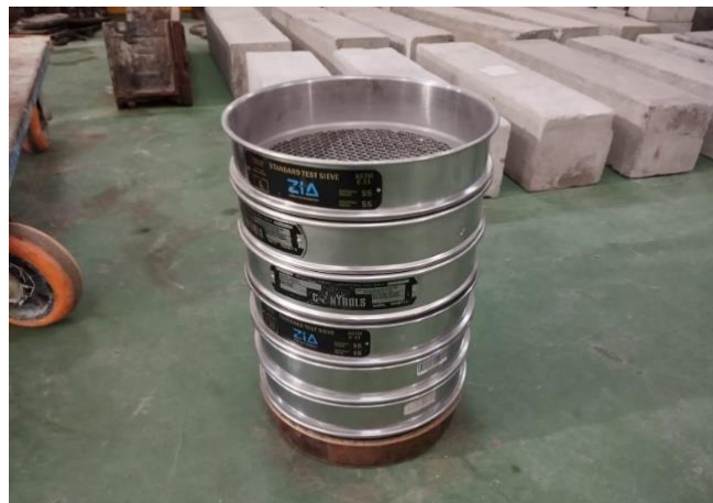
Gambar 3.2: Saringan agregat halus No. 4, No. 8, No. 16, No. 30, No. 50, No. 100, dan PAN.
