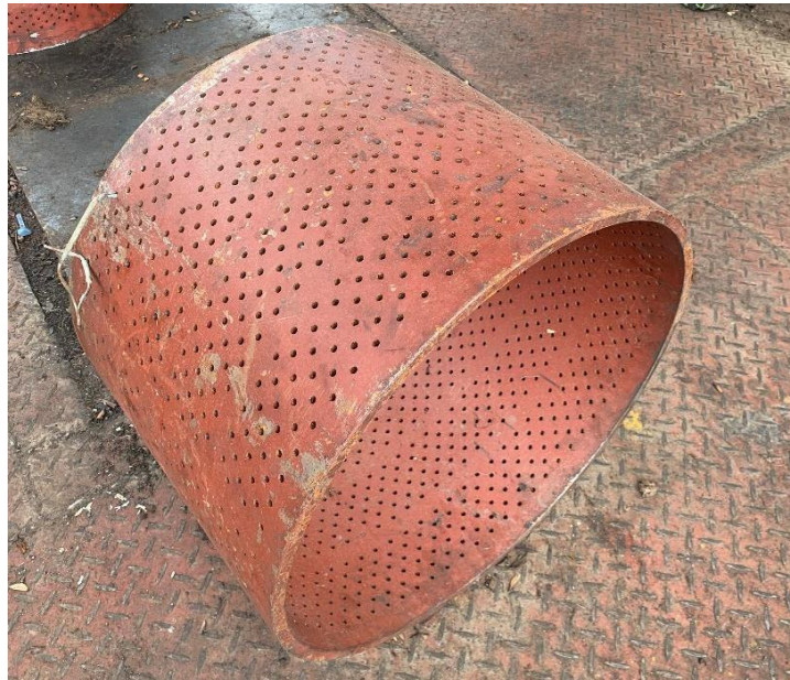
Gambar 2.10 Silinder/cage Berlubang (Ruang Press)
