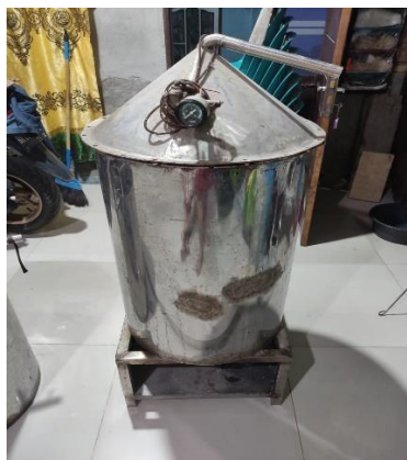
Gambar 3.4 Ketel Uap / Boiler
