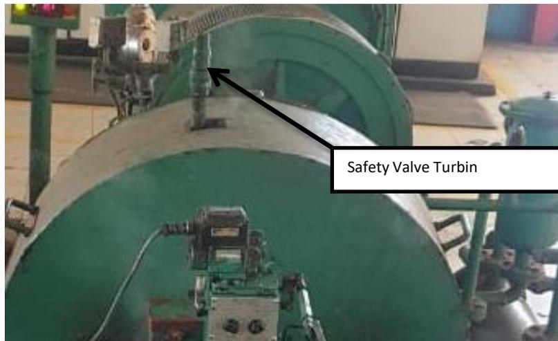
Gambar 2. 13 *Safety valve turbin*
