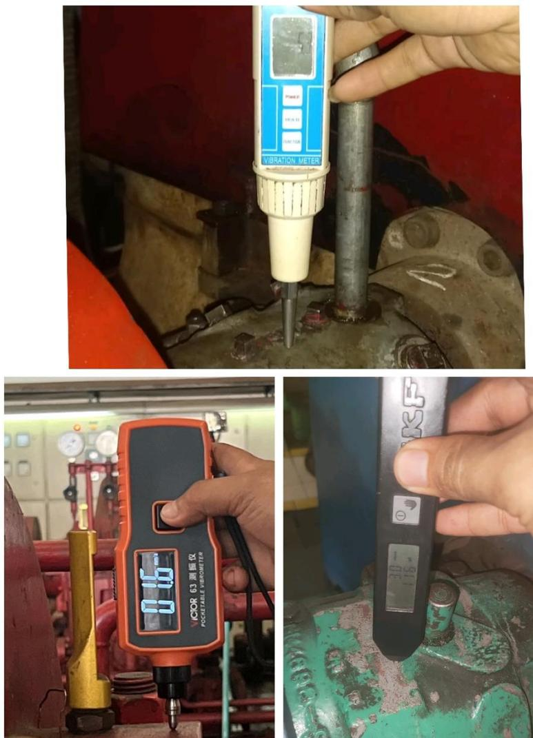
Gambar 2. 33 Alat Ukur Vibrasimeter
