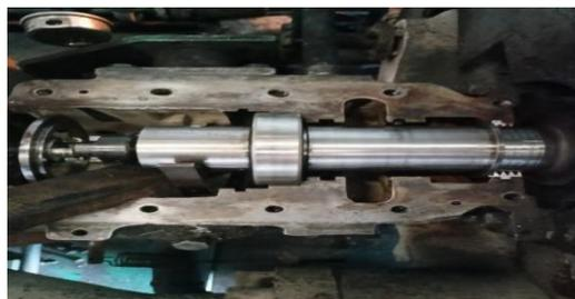
Gambar 2. 7 *Thrust Bearing*(Adibrata
