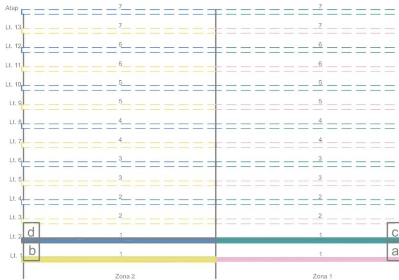
Gambar 4.4: Rotasi Material Bekisting Balok 2 Lantai.
