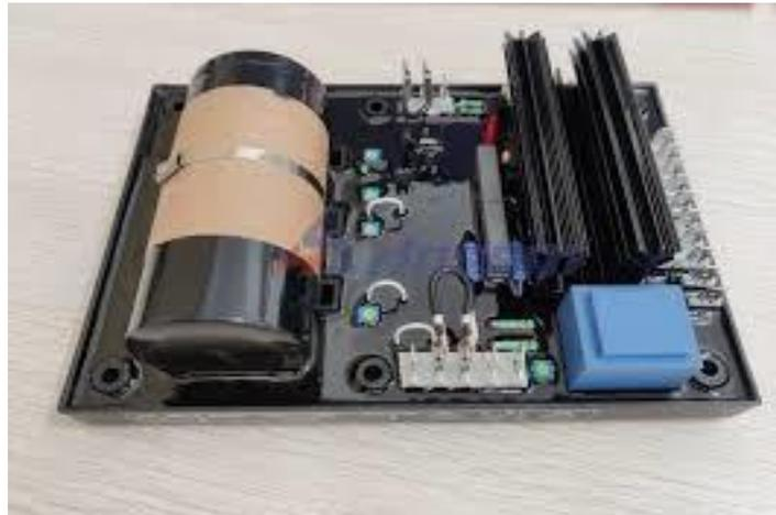
Gambar 2.5 *Automatic Voltage Regulator*
