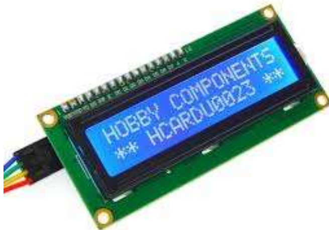
Gambar 3.9 LCD I2c 16x2
