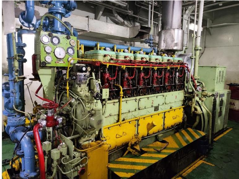
Gambar 2. 1 *Auxiliary Engine*
