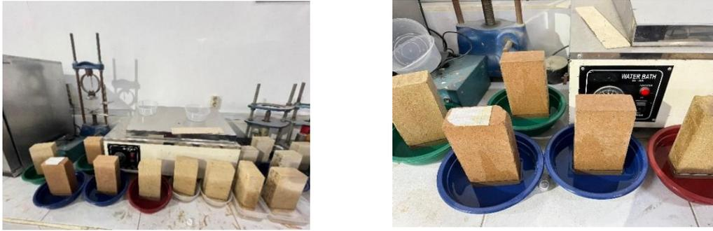
Gambar 4.16: Proses pengujian kadar garam.
