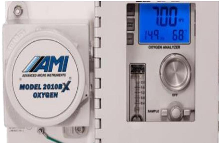
Gambar 2.15 O<sub>2</sub> Analyzer
