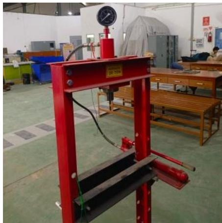
Gambar 3.8: Mesin hidrolik press.
