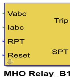
Gambar 4. 3 Blok Rele Jarak
