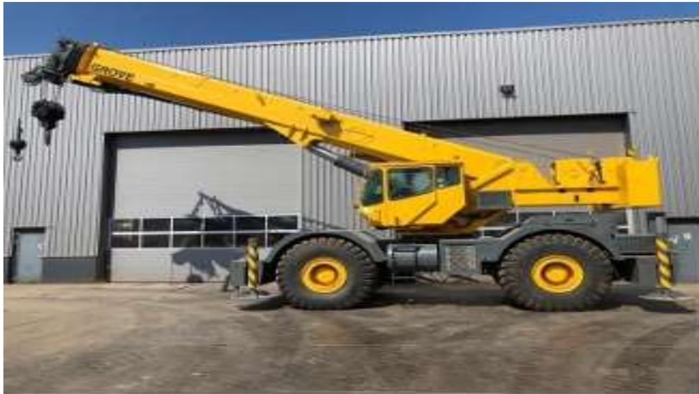
Gambar 2.2 *Rough Terrain Crane* (IMANULLAH, M. F, 2022)
