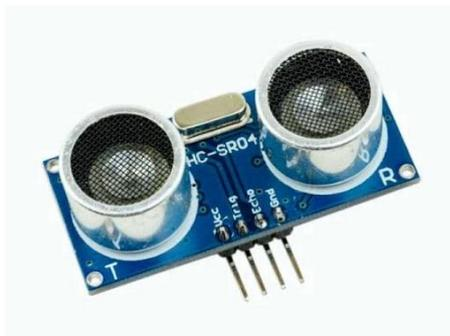
Gambar 2. 6 Sensor Ultrasonik
