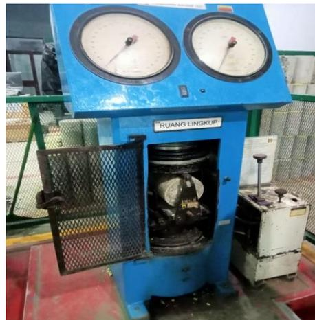
Gambar 3. 3: *Compression Testing Machine (CTM).*
