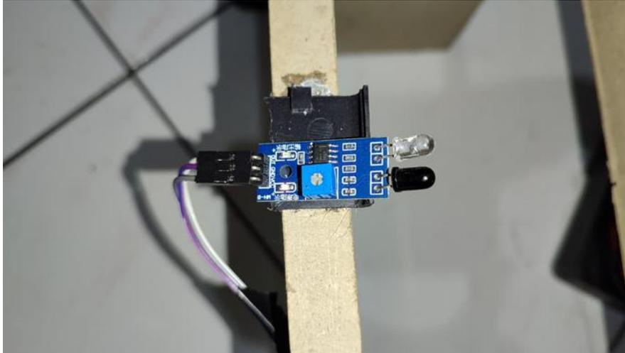
Gambar 4.2 Sensor *Obstacle Avoidance*
