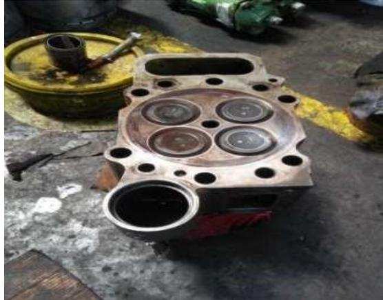
Gambar 2.6 *Cylinder Head* (PT. Waruna Shipyard Indonesia)2024
