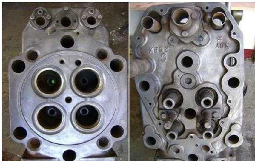
Gambar 3.1 *Cylinder Head* (PT Waruna Syipyard Indonesia)
