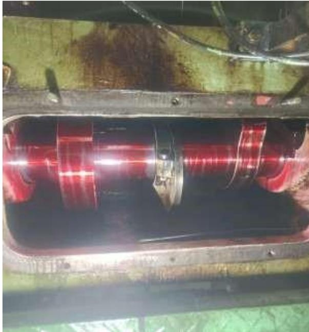
Gambar 2.17 Poros Nok (*Cam Shaft*) (PT. Waruna Shipyard Indonesia)2024
