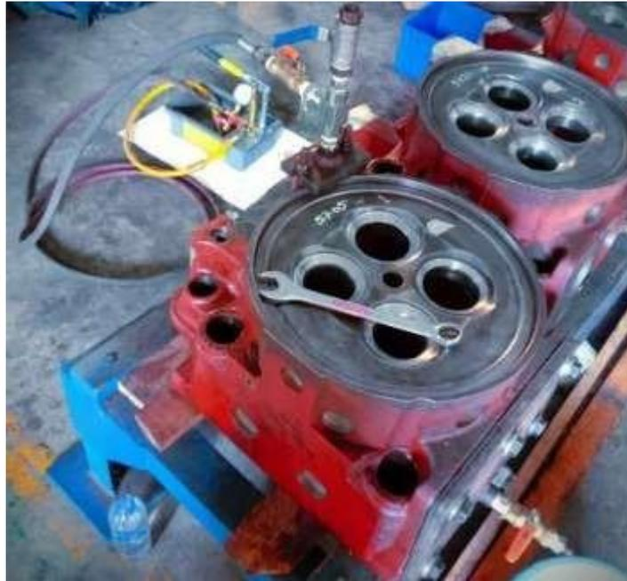
Gambar 3.4 *Test Press*
