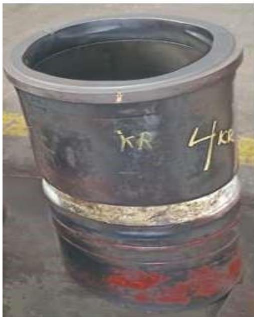
Gambar 2.5 *Cylinder Liner* (PT. Waruna Shipyards Indonesia)2024
