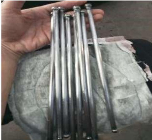
Gambar 2.11 *Push Rod* (PT. Waruna Shipyard Indonesia)2024
