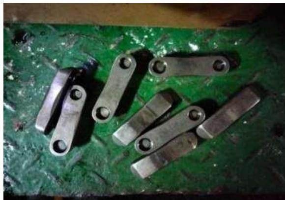
Gambar 2.16 *Crosshead* (PT. Waruna Shipyard Indonesia)2024
