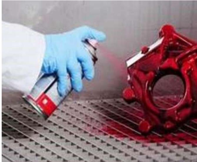
Gambar 3.3 *Dye Penetrant Test*
