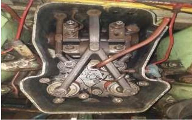
Gambar 4.1 Membongkar cover *Cylinder Head*
