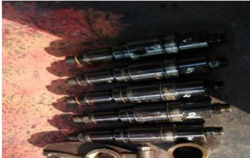
Gambar 2.9 Injector (PT. Waruna Shipyards Indonesia) 2024 6.
