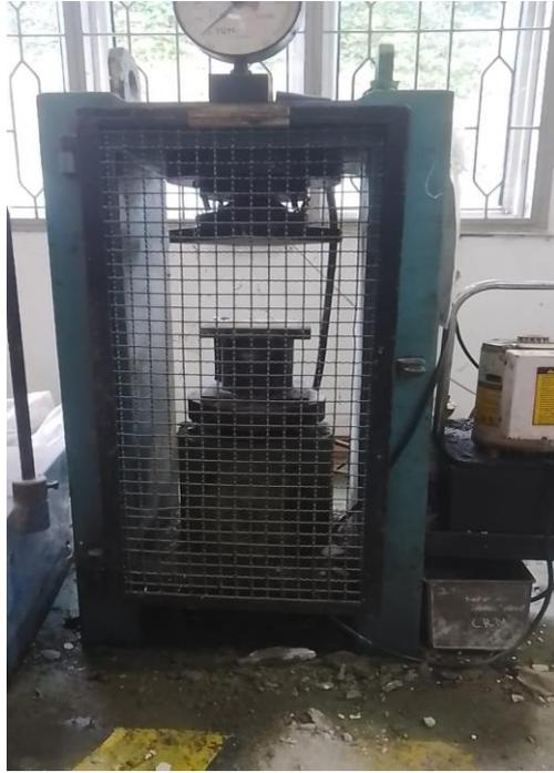
Gambar L- 1 *Compressing Test Machine*
