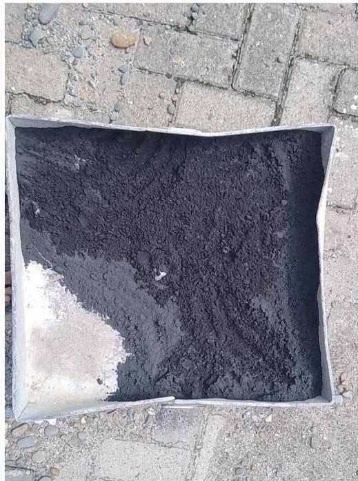
Gambar L- 4 Abu cangkang sawit
