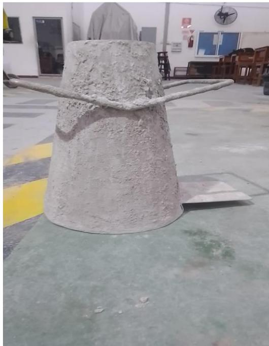
Gambar L- 8 Kerucut abrams
