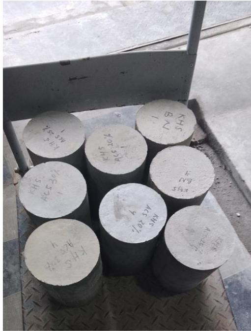
Gambar L- 11 Beton Campuran Variasi Abu Cangkang Kelapa Sawit
