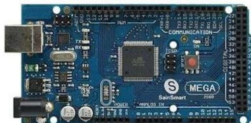
Gambar 2.8 Arduino Mega 2560
