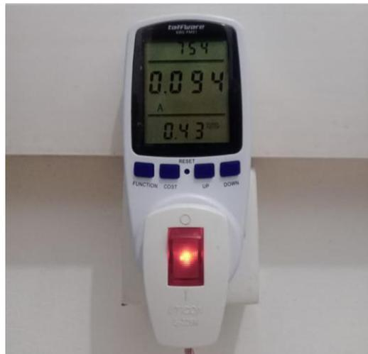
Gambar 3.9 Watt meter digital
