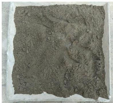
Gambar 3.23: Agregat halus lolos saringan no 4.
