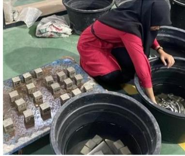
Gambar 3.110: Perendaman benda uji mortar
