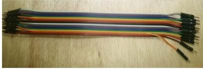
**4.5 Gambar kabel Jumper**
