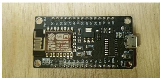
**4.4 Gambar NodeMCU ESP 8266**
