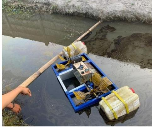
Gambar 4.23 Proses penelitian mesin *oil skimmer tipe drum roller*
