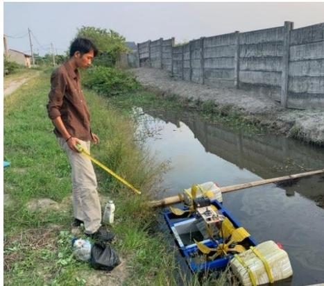
Gambar 4.21 Proses penelitian mesin *oil skimmer tipe drum roller*
