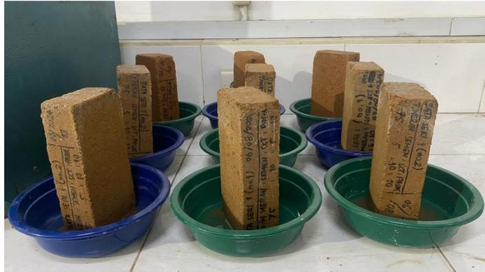
Gambar 4.16: Proses pengujian kadar garam.
