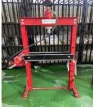
Gambar 3.3: Mesin hidrolik press.
