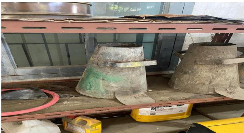
Gambar alat Slump Cone
