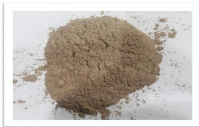
Gambar 2 3 : *Ladle Furnace Slag* (LFS)
