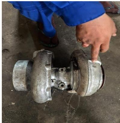
Gambar 4.4 *casing* turbin (PT.WSI)
