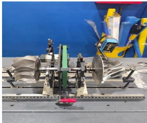
Gambar 4.31 *turbocharger* naik *balancing* (PT.WSI)
