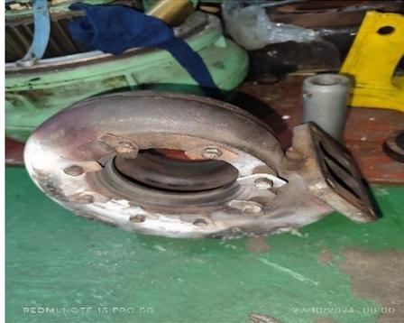
Gambar 2.6 *Casing* Turbin ( PT WSI 2024 )
