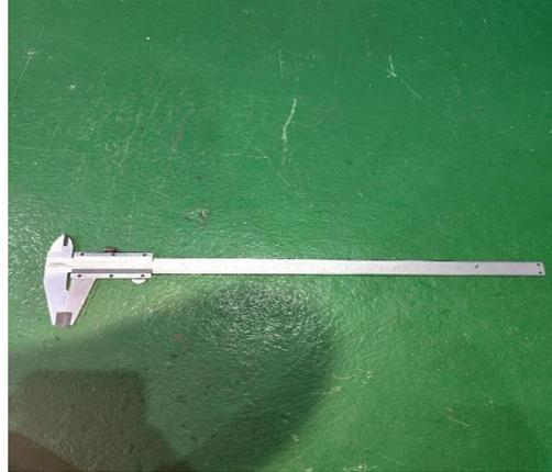
Gambar 3.8 Jangka Sorong (PT.Waruna Shipyard Indonesia )
