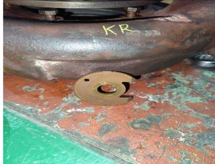
Gambar 4.9 *Thrust bearing* (PT.WSI)
