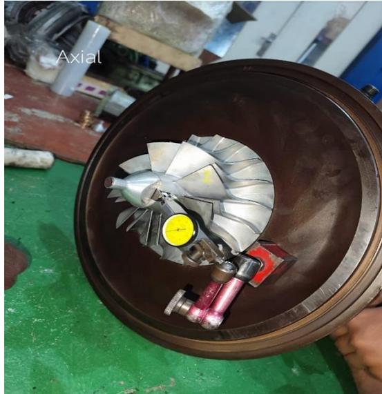
Gambar 3.10 *Dial Axial/Radial* (PT. Waruna Shipyard Indonesia )
