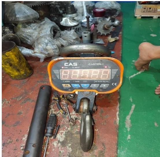
Gambar 3.9 Timbangan Digital (PT.Waruna Shipyard Indonesia )
