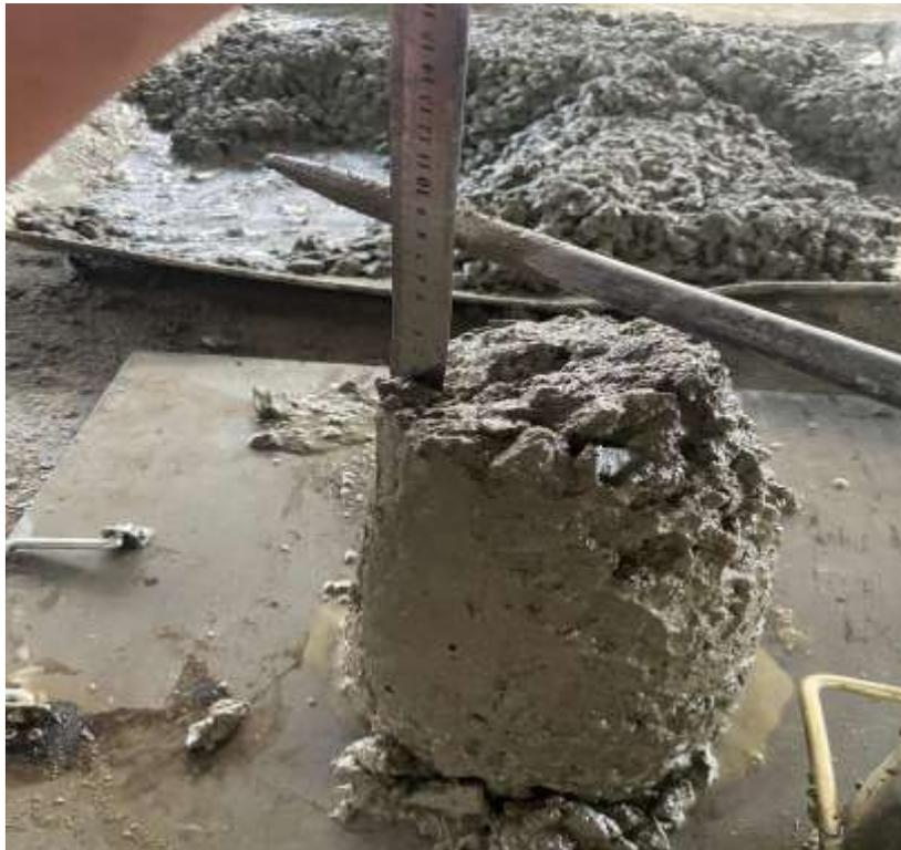
Gambar L.6: Pengujian *slump test*.
