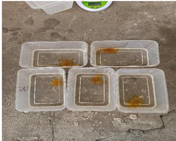
Gambar 4.3 Perendaman Serat Daun Nanas Dengan Variasi 1, 3, 5, 7, 9 Jam
