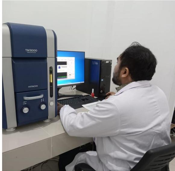
Gambar 4.4 Pengujian *Scanning Electron Microscope* (SEM)
