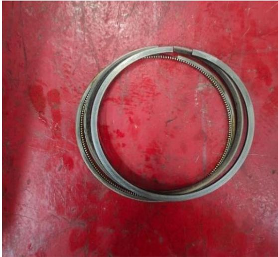
Gambar 2.7 Ring torak (Ring piston) (PT. Waruna Shipyards Indonesia)
