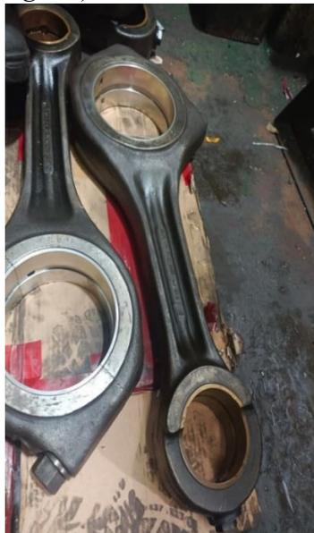
Gambar 2.8 Batang torak (*connecting rod*) (PT. Waruna Shipyards Indonesia)
