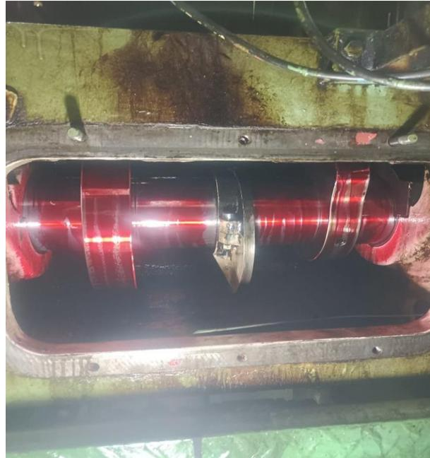
Gambar 2.13 Poros nok (*cam shaft*) (PT. Waruna Shipyard Indonesia)
