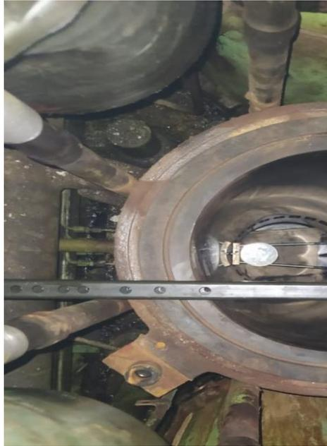
Gambar 4.20 Korosi *Cylinder Liner*
