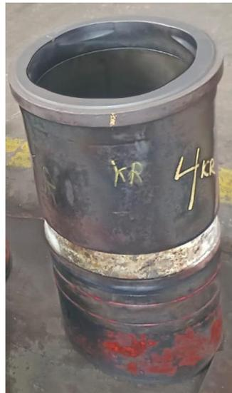
Gambar 3.1 *Cylinder Liner*
