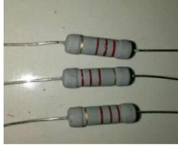
Gambar 3. 6 Resistor 4700 Ohm
