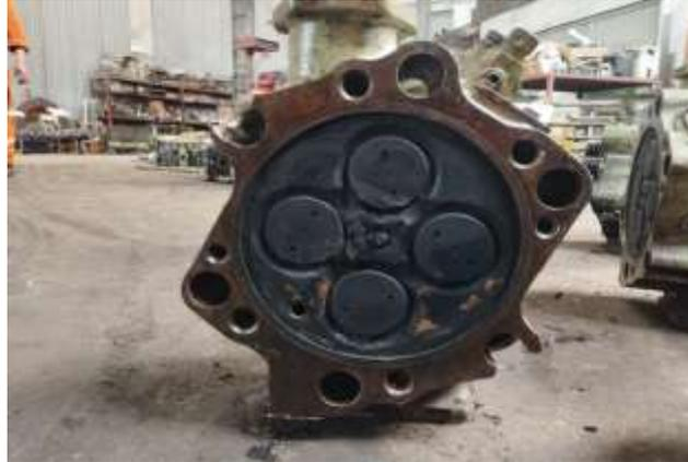
Gambar 2.4 *Cylinder Head* Mesin *Diesel*
