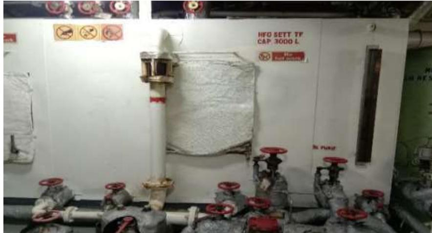
Gambar 2.16 *Settling Tank*
