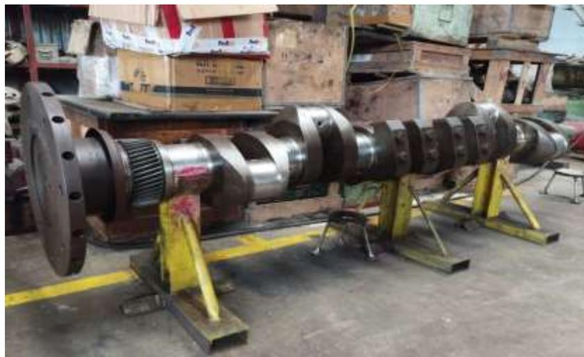
Gambar 2.8 Poros Engkol (*Crank Shaft*) Mesin Diesel
