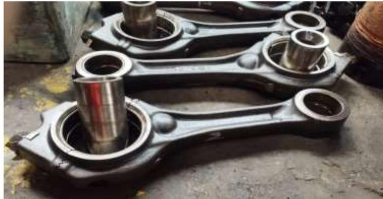
Gambar 2.7 Batang Engkol (*Connecting rod*) Mesin Diesel
