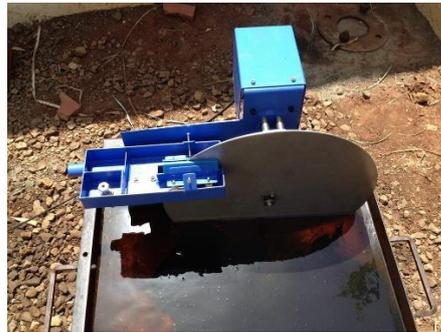
Gambar 2.3 Mesin *Oil Skimmer Tipe Disc* (Sumber [indiamart.com](http://indiamart.com))
