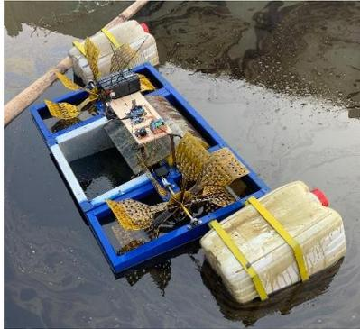
Gambar 3.5 Mesin *oil skimmer tipe drum roller* (Sumber Dokumentasi Pribadi)
