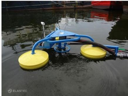
Gambar 2.5 Mesin *Oil Skimmer Tipe Weir* (Sumber [Elastec.com](http://Elastec.com))
