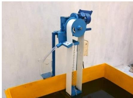
Gambar 2.2 Mesin *Oil Skimmer Tipe Belt* (Sumber [indiamart.com](http://indiamart.com))
