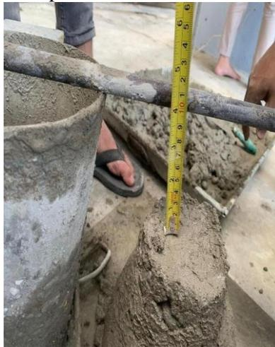
Gambar L-6 Pengecekan Nilai Slump
