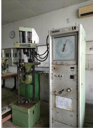
Gambar 2. 8 Mesin Uji Bending (Bending Test)
