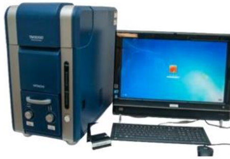
Gambar 3.9 Alat Uji Scanning Electron Microscope (SEM)
